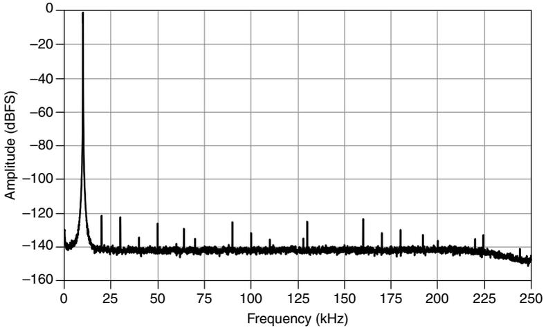
**Figure 6.** PCI-5922 Dynamic Performance with 10 kHz Input Signal, Measured, 1 M $\Omega$ , 2 V<sub>pk-pk</sub> Range, 100 kS/s, Unbalanced Differential, 10,000-Point FFT with 10 Averages
